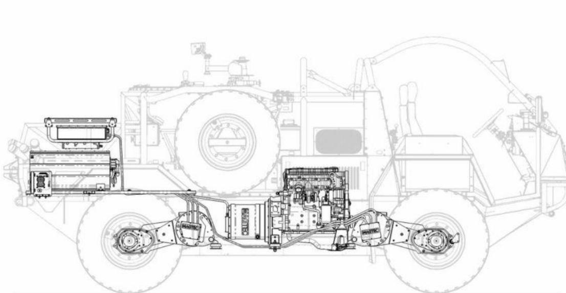
*Side drawing of the Jackal 1 4x4 hybrid electric drive, which has a Cummins four-cylinder diesel coupled to a Magtec generator. (Supacat)*
