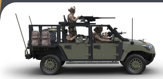
The Supacat Light Mobility Vehicle (LMV) combines proven COTS automotive components with a bespoke chassis and proven Combat cell to deliver a vehicle that is best in breed and uniquely modular and configurable to suit a wide variety of light roles.
